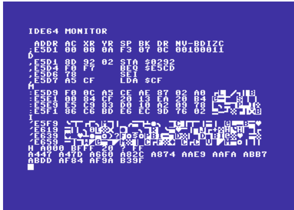
Figure 7: The IDE64 builtin monitor
