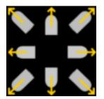
Force applied by a beam of 2 forces. This elements have similar characteristics of forces. The only difference is that if the data of the force is unknown, the result will display if the beam is in tension or compression. Since this element represent the force applied by the beam, a positive value means compression and a negative means tension.
