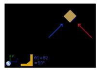
Our intention to introduce a frictional force is find the angle when the slip is imminent. Thus, the block element represents the point where is applied the normal and here we apply the friction force too (we can move the friction along its action line, so we can apply it in this element).
